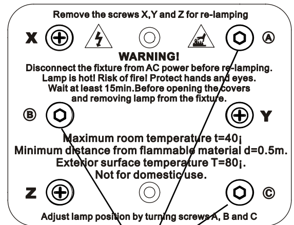
3 adjustment screws "A,B,C"
